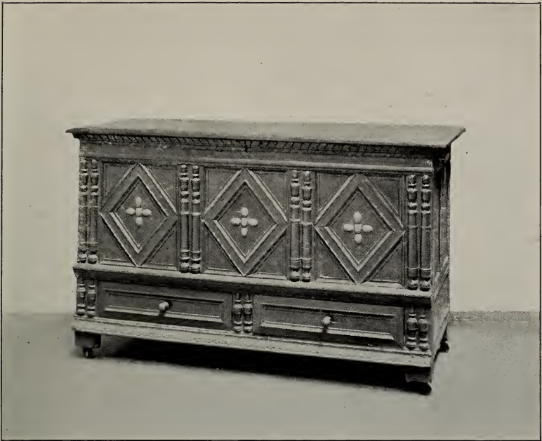
Chest of Miles Standish. An interesting decorative treatment utilizing woodturning and paneling on a box construction. Note that in no instance does decoration seek to hide construction.
